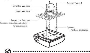
**Note:** It is recommended that you keep a reasonable space between the bracket and the projector to allow for proper heat distribution. Use two washers for extra support, if deemed necessary.
