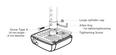
5 Adjust the angle and positioning as necessary.
