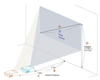
The table below shows how to achieve a desired image size by adjusting either the position or the zoom ring. For example: to obtain an image size of 50" set the projector at a distance 1.7 m and 1.8 m from the screen and adjust the zoom level accordingly.
