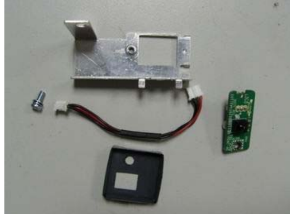
Disassemble the back IR assy.
