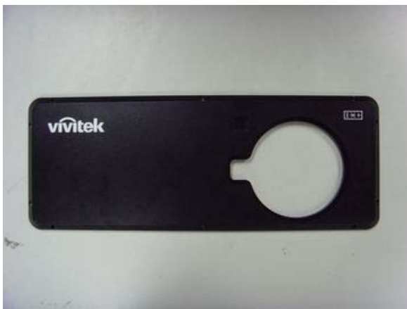
Remove the front cover.
