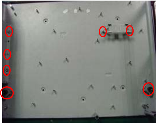
Remove these screws and take away the three parts.
