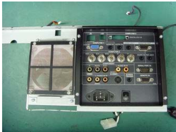
Then remove the IO BD Assy.
