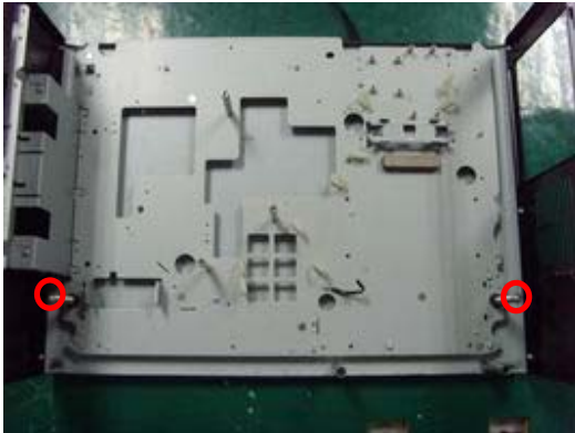
Remove the two screws and take away the ADJ foot.
