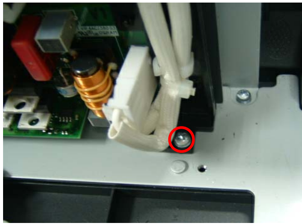
Remove the screw
