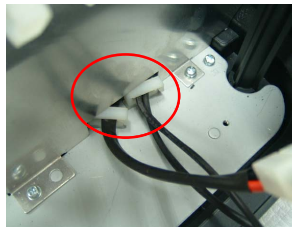
Arrange the wires as picture when you assemble it.
