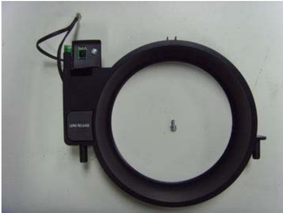
Disassemble the Lens cap & IR Assy.
