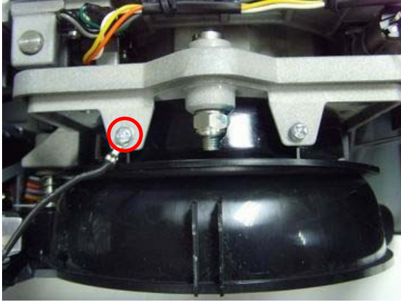
Remove the screw.
