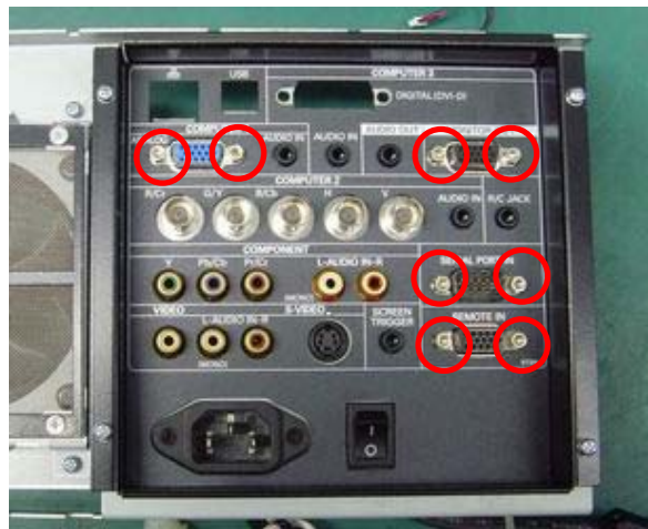
Remove the eight hexagonal bolts.
