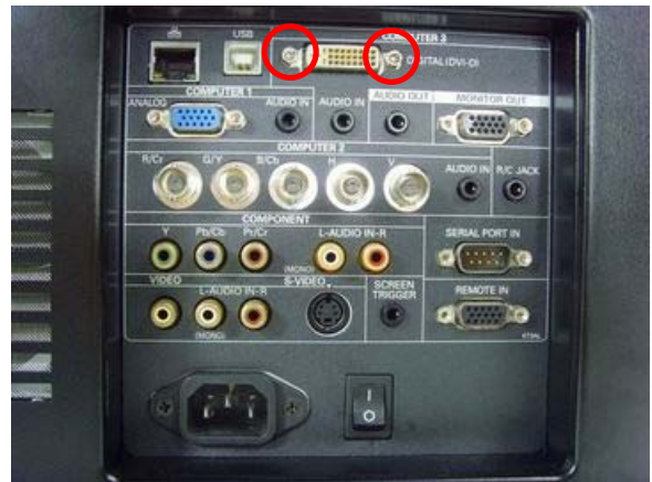
Remove the two hexagonal bolts then take off the main BD.
