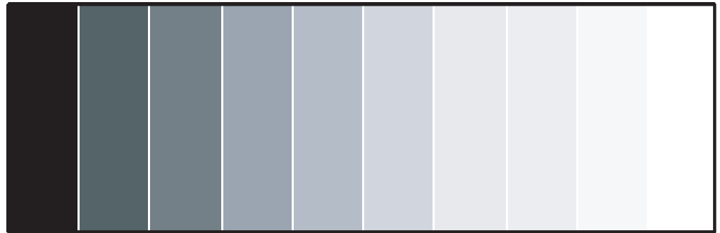
Figure 4-3. Typical Gray Bar Pattern for Adjusting Contrast
