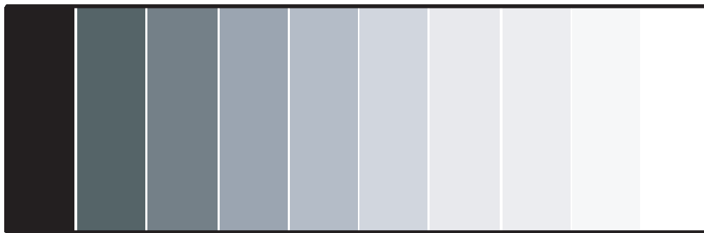
Figure 4-3. Typical Gray Bar Pattern for Adjusting Contrast
