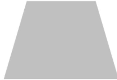
From the projector, the image path is shorter along the top.
