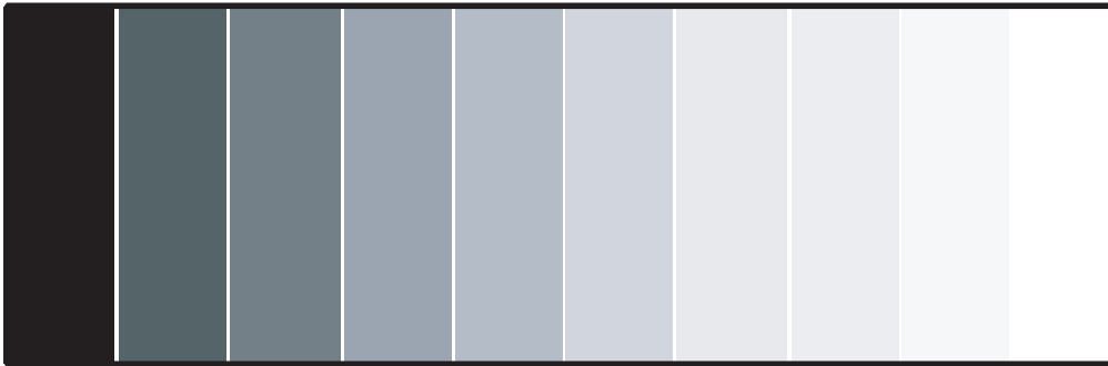
Figure 4-3. Typical Gray Bar Pattern for Adjusting Contrast
