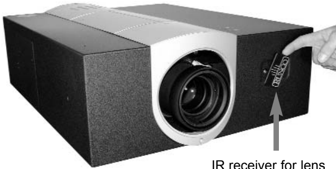
IR receiver for lens zoom / focus motors
