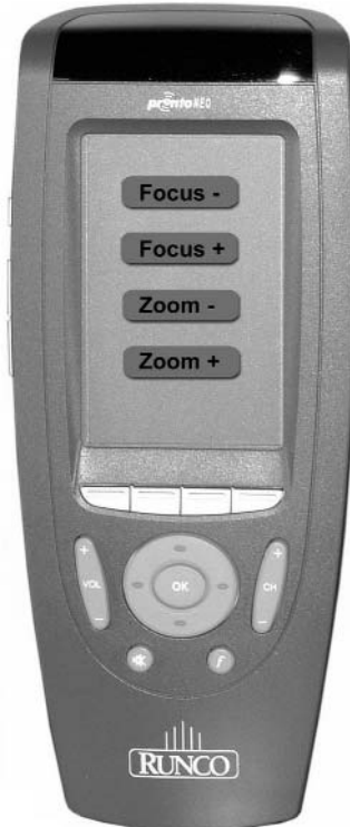
Focus & Zoom Screen: This screen allows you to access the focus and zoom feature.
