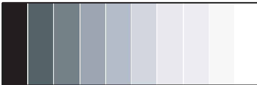
Figure 3-9. Typical Gray Bar Pattern for Adjusting Contrast
