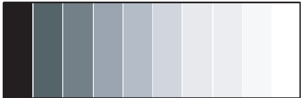
Figure 4-3. Typical Gray Bar Pattern for Adjusting Contrast
