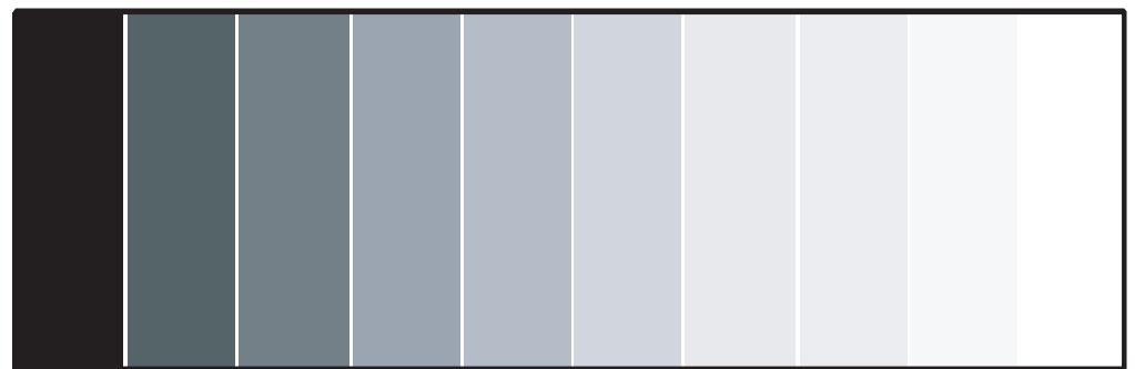
Figure 4-4. Typical Gray Bar Pattern for Adjusting Contrast
