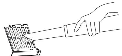
4. Place and slightly slide in the **Air filter** in the **Air intake port** to attach.
