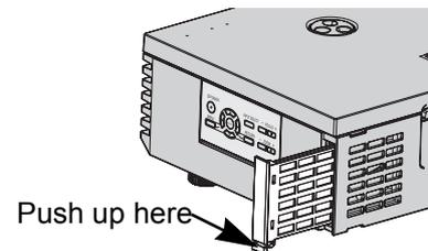
3. Vacuum dirt and dust from the **Air filter**.
