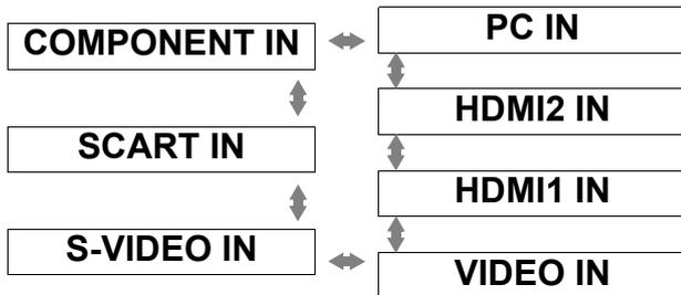
Graphical guidance will be displayed on the upper right of the display and you can confirm the selected input method which is highlighted in yellow. See "INPUT GUIDE" on page 38.
