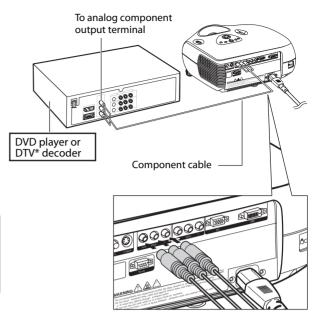
The device's component jacks may be labeled Y, CB and CR. Connect each jack as shown below.
