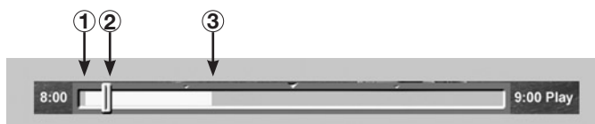
Figure 14. TV Pause slider. 1. Limit of backward scan. 2. Current viewing point in recorded portion of program. 3. Current broadcast point (limit of forward scan)
