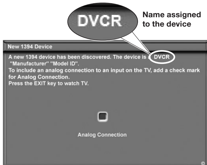
Figure 3. The ClearThought Auto Input Sensing screen for IEEE 1394 devices includes a check box for an associated analog connection.
