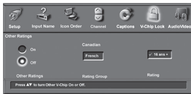
Figure 12. The Other Ratings menu is available only if the TV receives broadcast signals carrying an alternative rating system.
