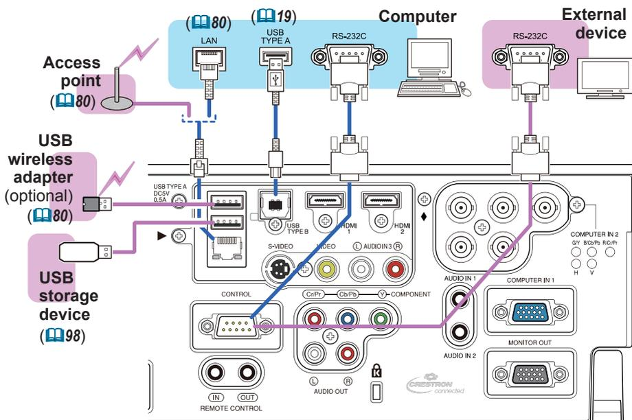
**⚠ WARNING** ▶ Heat may build up in the USB wireless adapter, to avoid possible burns disconnect the projector power cord for 10 minutes before touching the adapter.
