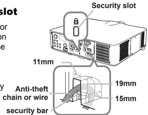
**⚠ WARNING** ▶ Do not use the security bars and slot to prevent the projector from falling down, since it is not designed for it.
