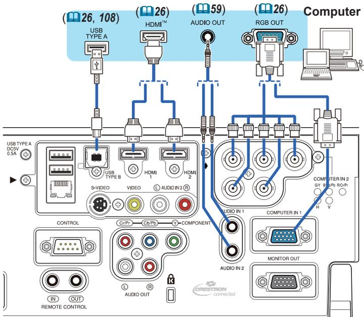
**NOTE** • Before connecting the projector to a computer, consult the computer's manual and check the compatibility of the signal level, the synchronization methods and the display resolution output to the projector.
