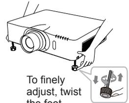
To finely adjust, twist the foot.
