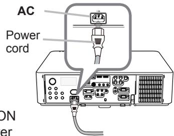
Please remember that when the **DIRECT POWER ON** function activated (69), the connection of the power supply make the projector turn on.
