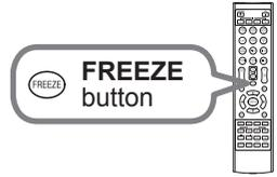
**NOTE** • The projector automatically exits from the FREEZE mode when some control buttons are pressed.
