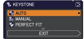
**NOTE** • The menu or dialog will automatically disappear after several seconds of inactivity. Press the **KEYSTONE** button again, or point the cursor at EXIT in the dialog and press the ► or **ENTER** button to end the operation and close the menu or dialog.
