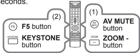
Please remember that the REMOTE FREQ. in the SERVICE item of the OPTION menu (🔧74) of the projector to be controlled should be set to the same mode as the remote control.
