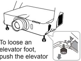
To loose an elevator foot, push the elevator button on the same side as it.
