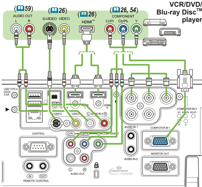
**NOTE** • The **HDMI** ports of this model are compatible with HDCP (High-bandwidth Digital Content Protection) and therefore capable of displaying video signals from HDCP compatible DVD players or the like.
