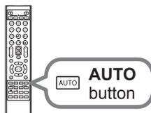
**NOTE** • The automatic adjustment operation requires approx. 10 seconds. Also please note that it may not function correctly with some input.
