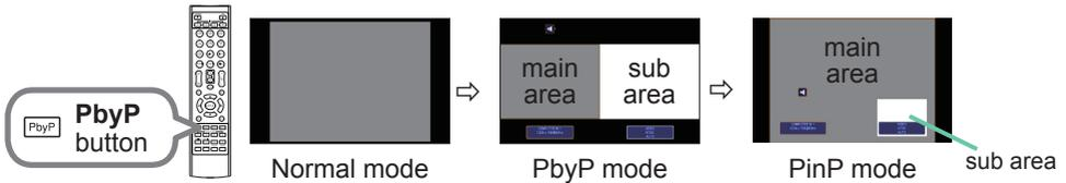
Press the **PbyP** button on the remote control. This activates the PbyP mode. Then, press the **PbyP** button again. The projector goes into PinP mode. The screen displayed before the **PbyP** button was pressed will be displayed as the main area. Most of operations are effective for the main area only. Only outputs the audio input signal paired with the picture input signal for the main area. To quit the PinP mode, press the **PbyP** button again.
