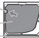
**⚠ WARNING** ► Before taking care of the air filter, make sure the power cable is not plugged in, then allow the projector to cool sufficiently.
