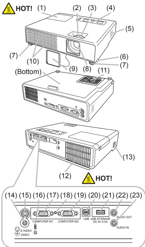
**⚠️ WARNING ► HOT! :** Do not touch around the lamp cover and the exhaust vents during use or just after use, since it is too hot.
