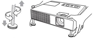
To finely adjust, twist the foot.
