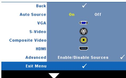
**AUTO SOURCE**—Select **Off** (the default) to lock the current input signal. If you press the **Source** button when the **Auto Source** mode is set to **Off**, you can manually select the input signal. Select **On** to auto detect the available input signals. If you press the **Source** button when the projector is on, it automatically finds the next available input signal.
