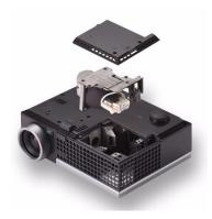
9 Reset the lamp usage time by selecting "Yes" for Lamp Reset in the OSD Lamp tab (see Lamp menu on page 32). When a new lamp module has been changed, the projector will automatically detect and reset the lamp hours.
