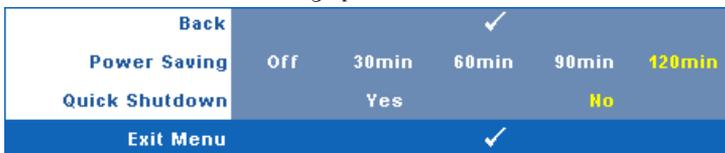
**POWER SAVING**—Select **Off** to disable Power Saving mode. By default, the projector is set to enter power saving mode after 120 minutes of no activity. A warning message appears on screen showing a 60-second countdown before switching to power saving mode. Press any button during countdown period to stop power saving mode.
