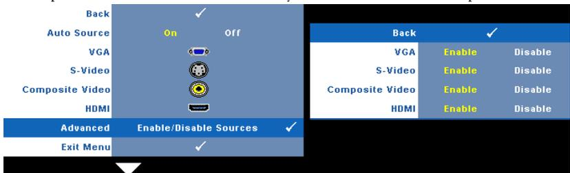
**VGA**—Use  and  to enable or disable VGA input.
