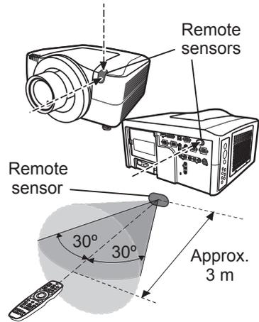
**NOTE** • You can inactivate one or two sensors from the three sensors using the item REMOTE RECEIVE. of the SERVICE menu under the OPTION menu.
