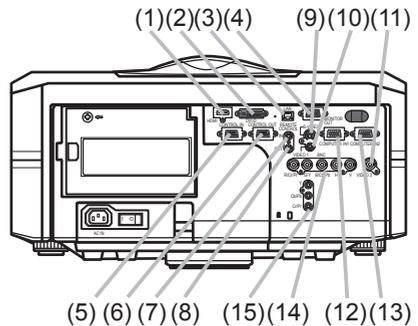
**⚠ CAUTION** ▶ Use the shutdown switch only when the projector is not turned off following the normal procedure, since pushing this switch stops operation of the projector without cooling it down.
