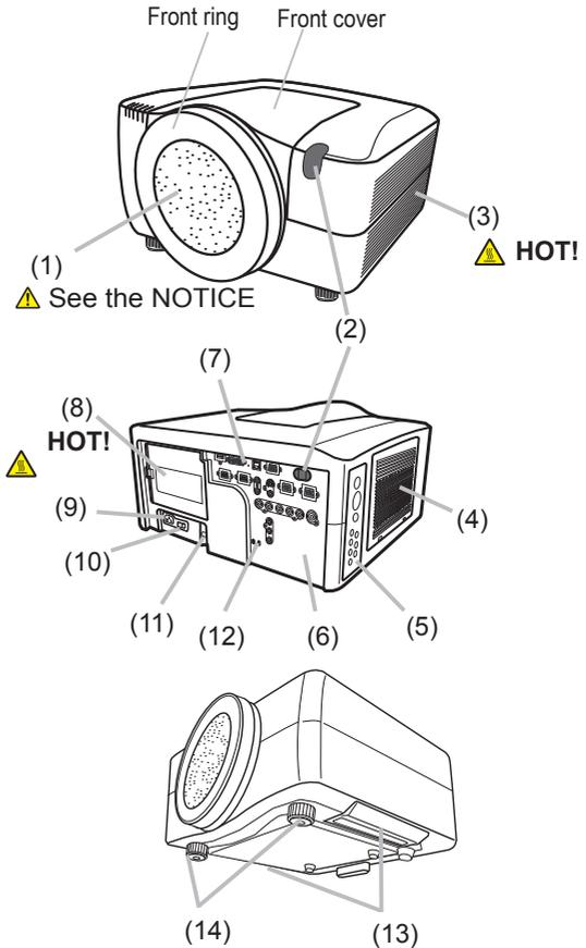
**⚠ WARNING ▶HOT! :** Do not touch around the lamp cover or the exhaust vents during use or just after use, since it is hot.
