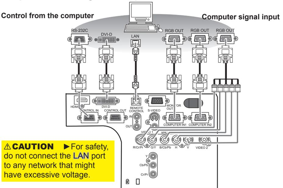
**⚠ CAUTION** ▶ For safety, do not connect the LAN port to any network that might have excessive voltage.
