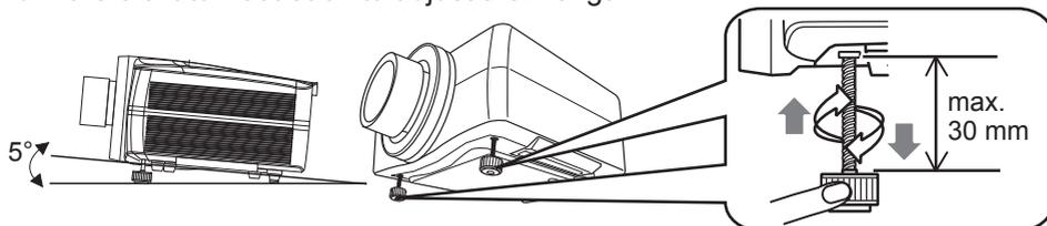
**⚠ WARNING** ▶ Do not lengthen the elevator feet to 30 mm or more. The foot lengthened exceeding the limit may come off and drop the projector down, and result in an injury or damaging the projector.
