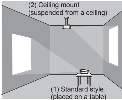
**NOTE** • In the case of ceiling mount, upward projection, or downward projection, the specified mounting accessories and service are required to install the projector. Request them from your dealer. Ask your dealer for installation other than styles above.
