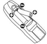
**NOTE** • If the remote control malfunctions, try replacing the batteries with fresh ones.
