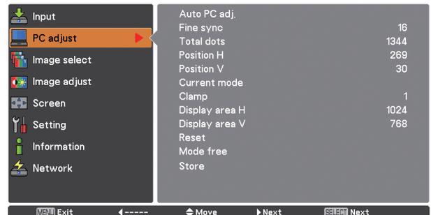
Use the Point ▲▼ buttons to select "Auto PC adj." and press the SELECT button. Please wait... appears while the Auto PC adjustment is in process.
