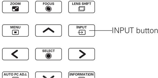
The input source changes each time you press the INPUT button on the side control as follows:
