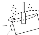
When hanging the projector from the ceiling, clean the air intake vent and top of the projector periodically with a vacuum cleaner. If you leave the projector unclean for a long time, the cooling fans can be clogged with dust, and it may cause a breakdown or a disaster.
