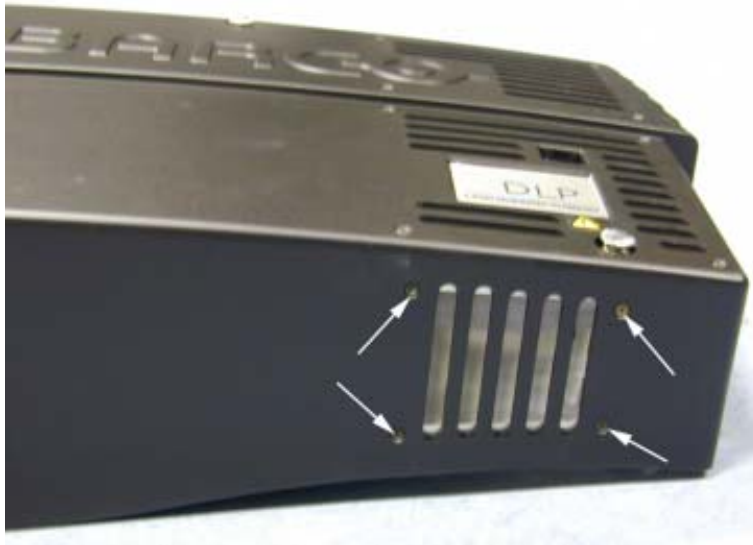
Image B-8 Dust filter removal
