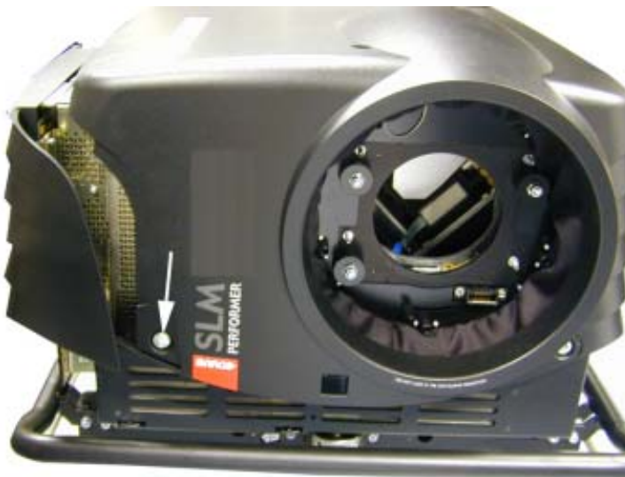
Image B-3 Front screw top cover removal
