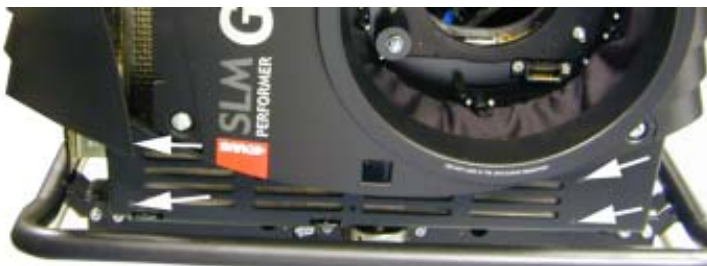
Image B-4 Dust filter removal
