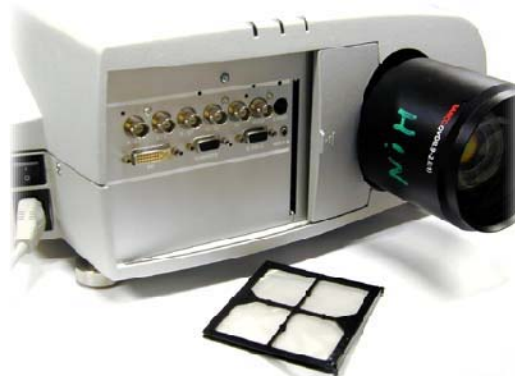
Image C-6 Input filter removed
