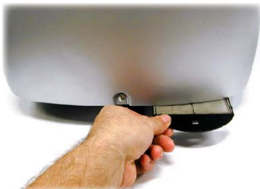
Image 13-3 Lamp filter removal
