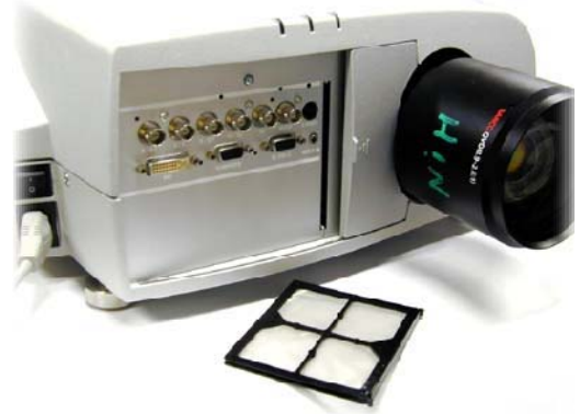
Image 13-6 Input filter removed
