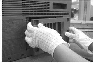
3 Remove the screw securing the Lamp by using a screwdriver.
