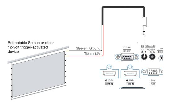
Figure 3-13. 12-Volt Trigger Output Connection
