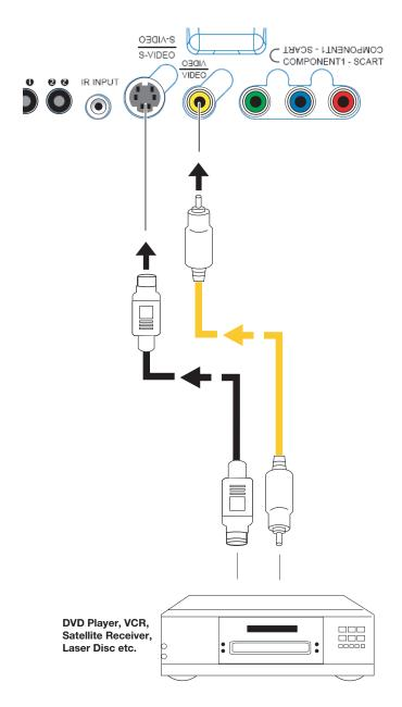
Figure 3-11. Composite and S-Video Connections
