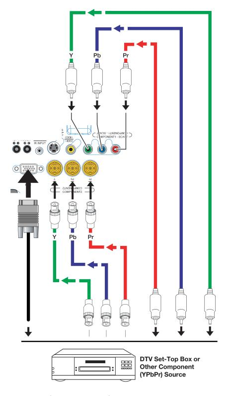
Figure 3-10. Component Video Connections
