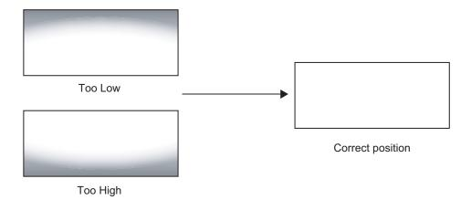
4. Then, adjust the anamorphic lens angle so that the projected image is rectangular:
