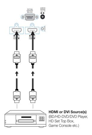
Figure 3-8. HDMI/DVI Source Connections
