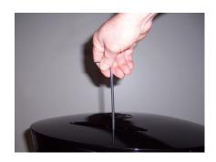
Horizontal Lens Shift (LS-5 only): To shift the projected image horizontally, insert the provided hex wrench into the hole at the top of the projector. Then, turn the wrench as shown to shift the lens in the desired direction.
