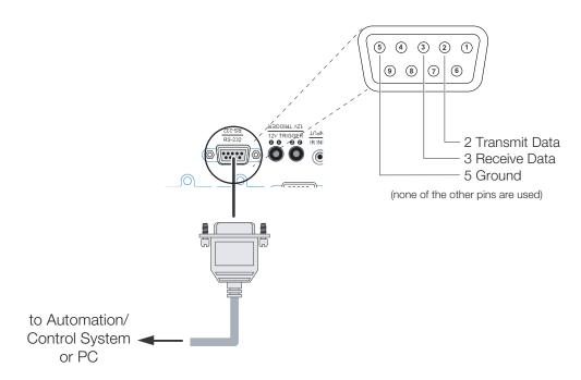
Figure 3-12. RS-232 Control System Connection
