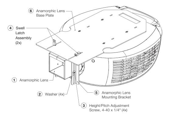
Figure 3-15. Anamorphic Lens Mounting Assembly - Exploded View
