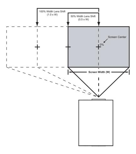
**Note:** This is a general example of lens shift. Lenses vary in their shift capabilities. **No particular lens or projector is used in this example.**
