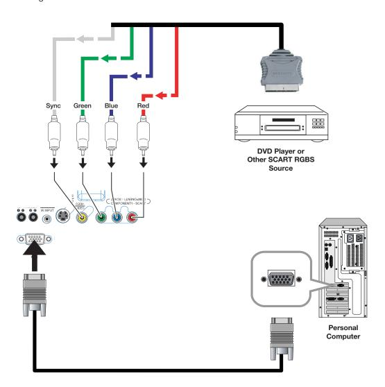
Figure 3-9. RGB Connections
