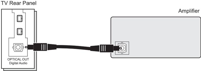
1) Connect the optical cable from the back of the TV to the back of the amplifier.
