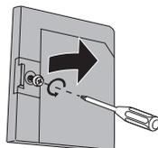
**Note:** Depending on which television you have, the lamp cover type shown to the right may be attached. If this is the case, you can loosen the screw located on the lamp cover by using your fingers, without the use of a Philips screwdriver (cross-head type). If the screw is difficult to loosen with your fingers, gently use a coin to loosen.
