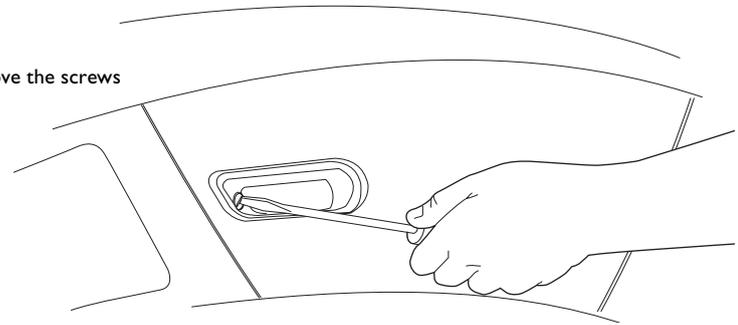
**4** Remove the lamp door by unscrewing the screw then sliding the door off.
