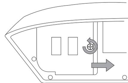
loosen 2 screws and remove
